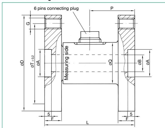
**Model 8628, torque sensor for static and dynamic applications, non-rotary**
