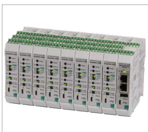
Fieldbus controller 9251 with up to 8 instrumentation amplifiers 9250
